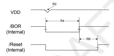
Figure 21-13. Software Reset Timing
