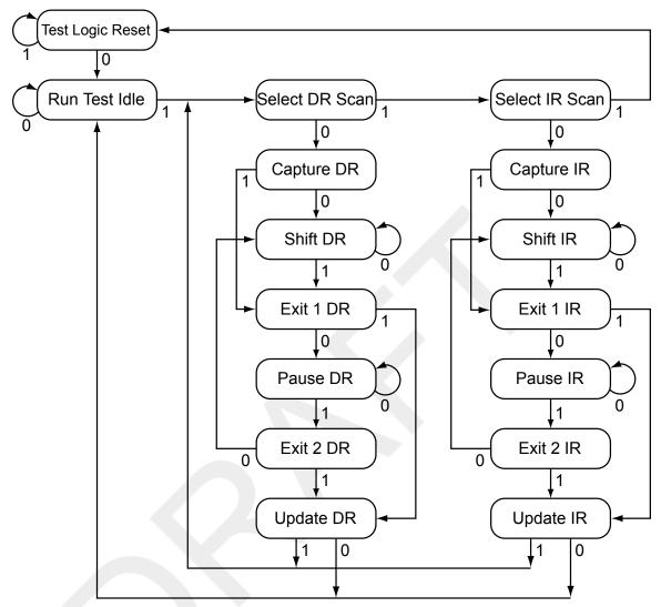
Figure 5-2. Test Access Port State Machine
