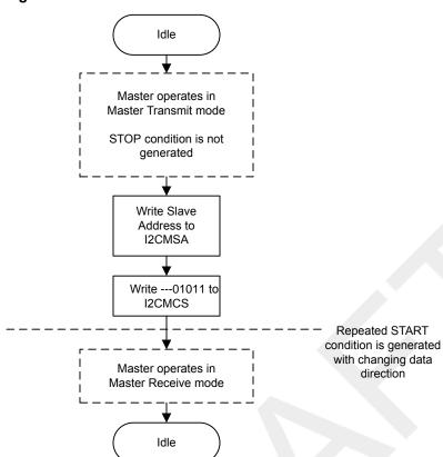
Figure 14-11. Master Burst RECEIVE after Burst SEND
