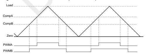
Figure 16-4. PWM Generation Example In Count-Up/Down Mode
