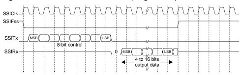
Figure 13-10. MICROWIRE Frame Format (Single Frame)
