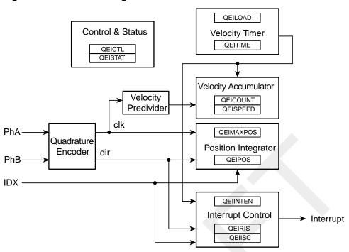
Figure 17-1. QEI Block Diagram
