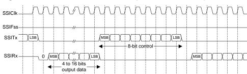
Figure 13-11. MICROWIRE Frame Format (Continuous Transfer)
