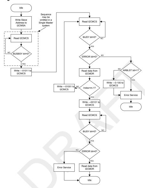
Figure 14-10. Master Burst RECEIVE
