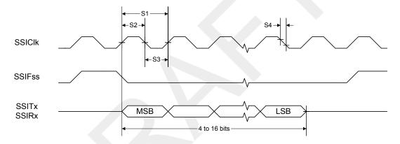
Figure 21-5. SSI Timing for MICROWIRE Frame Format (FRF=10), Single Transfer
