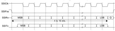
Figure 13-7. Freescale SPI Frame Format (Single Transfer) with SPO=1 and SPH=0
