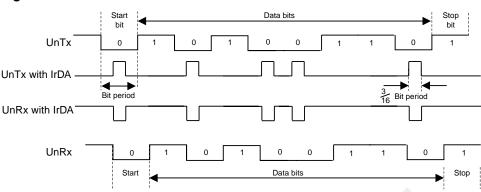
Figure 12-3. IrDA Data Modulation
